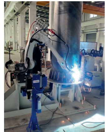
Mast robot welding for heliostats or trackers
