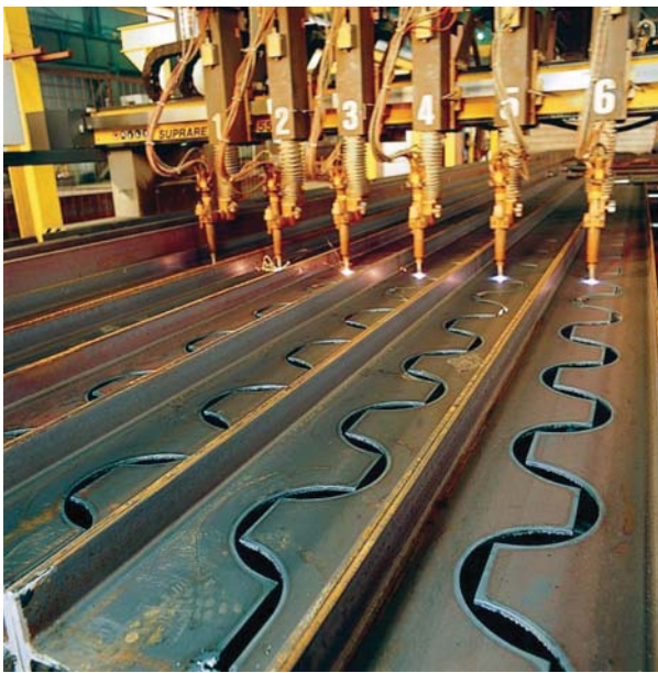
Figure 24: Cutting rolled sections for the manufacturing of ACB beams
