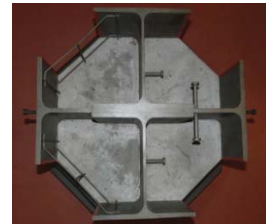
Composite column: box section welded from three sections encased in concrete
