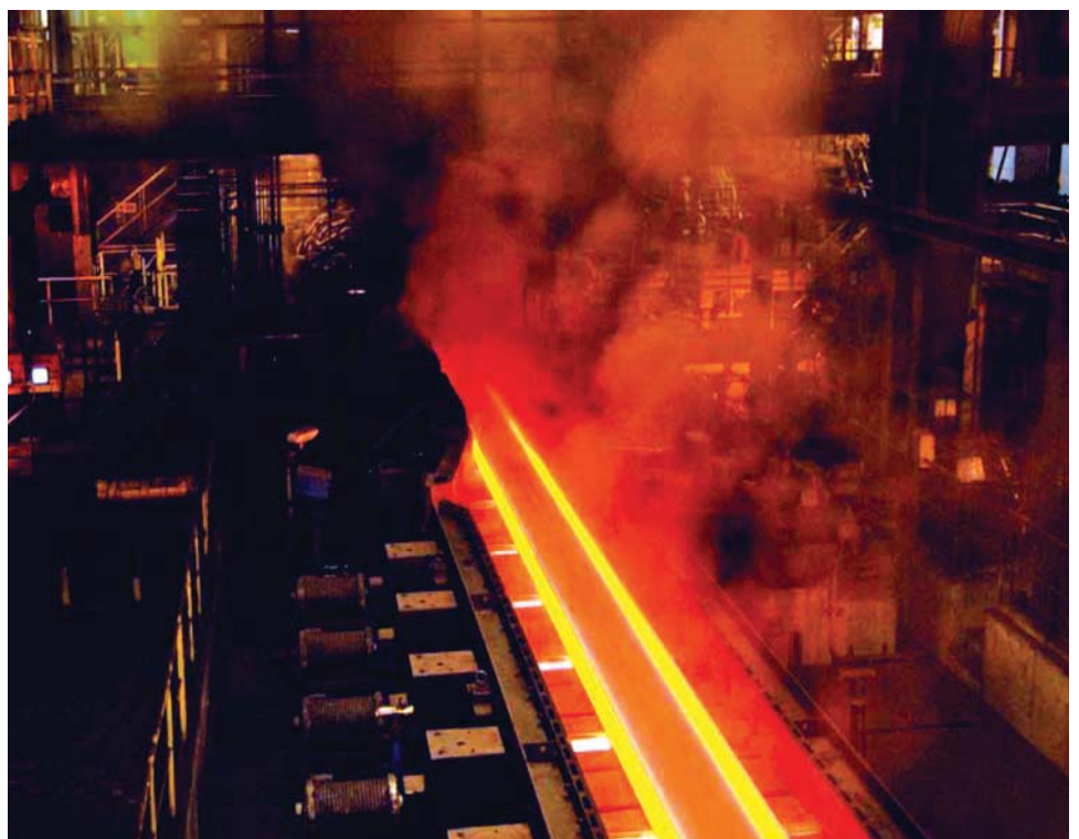
Figure 8: Rolling of a H1STAR-grade beam on the Grey rolling mill of ArcelorMittal in Differdange, Luxembourg
