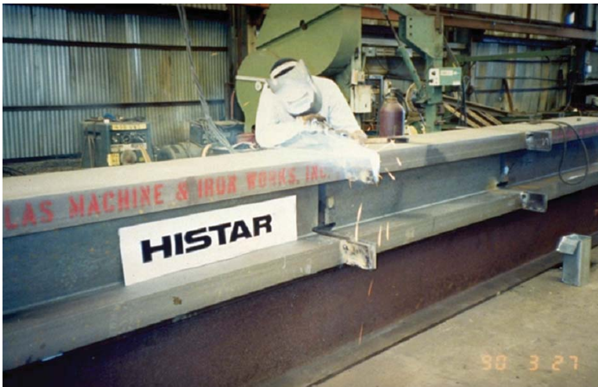
Figure 20: Welding of an HD 400 x1086 section made of HISTAR 460
