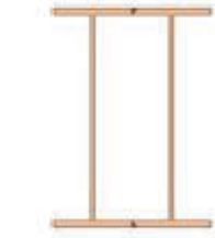
Box section welded from two sections
