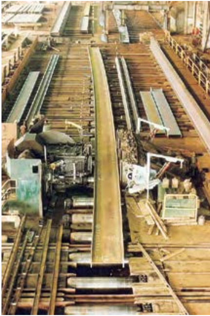
Finishing workshop - Cambering of bridge girders on the press.
