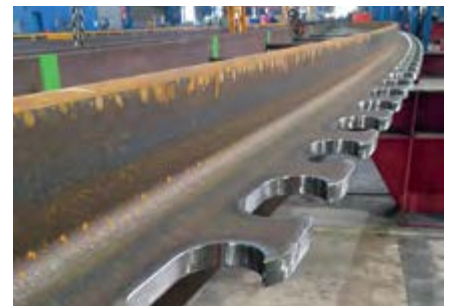
Precambering of a PreCoBeam in the finishing shop of ArcelorMittal.
