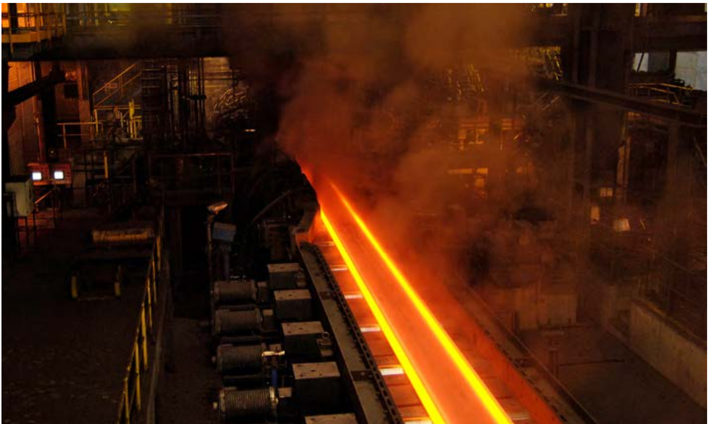
Rolling of a HISTAR® beam in the rolling mill of Differdange, Luxembourg
