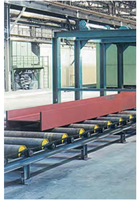
Automatic surface treatment equipment - Shot blasting and protective coating of beams.
