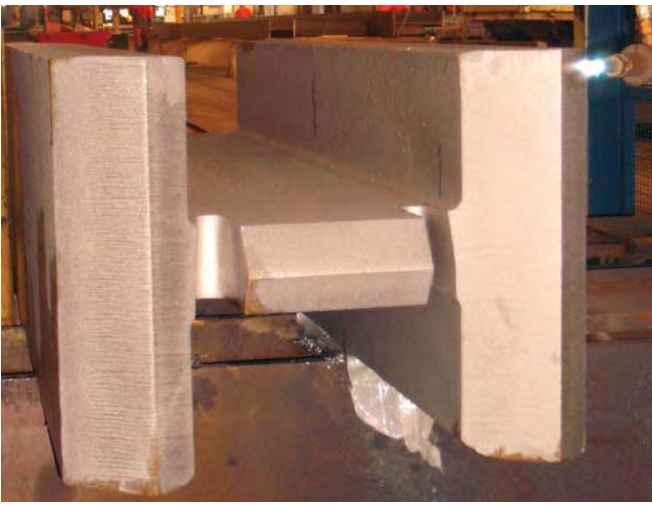
Figure 7.12: Bevel preparation on Jumbo
