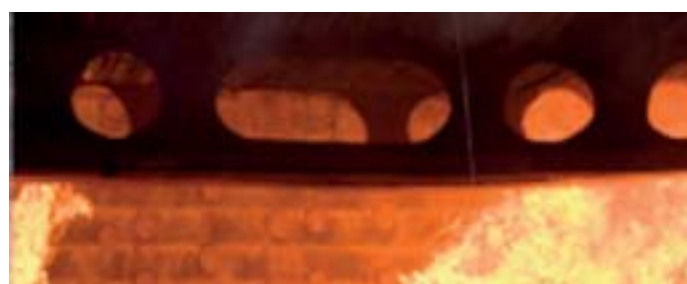
Figure 9.5: Fire test on unprotected cellular beams (FRACOF)
