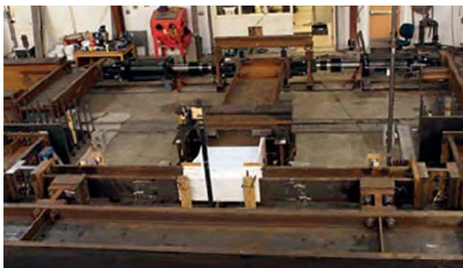
Figure 7.16: Specimen in testing orientation with two actuators.
