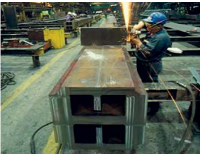
Figure 4.3: HD Box, made from 2 HD
