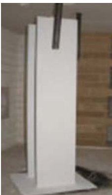
Figure 9.1: Intumescent coating layer
