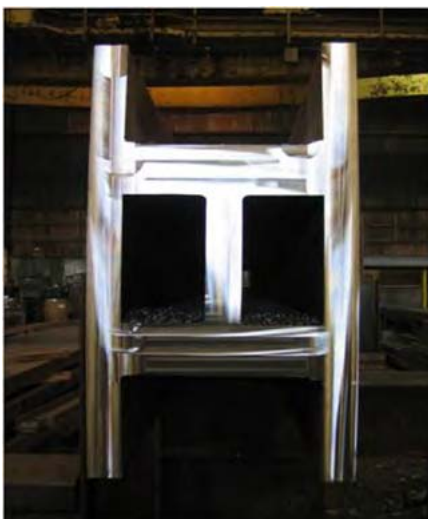
Figure 4.5: Rolled section with coverplates
